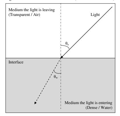
Figure 1. An illustration of refraction (with vertical normal)
